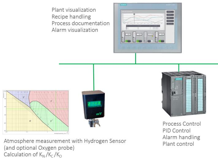
The system visualization, editing of the recipes, the process documentation and the visualization of faults are made available on the control panel.
